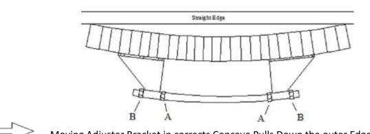
Moving Adjuster Bracket in corrects Concave Pulls Down the outer Edge
