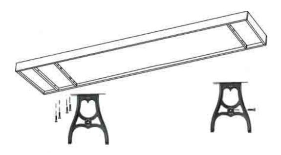
Attach stretcher with two bolts #4 no washers are used
