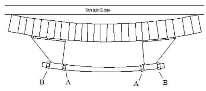
Moving Adjuster Bracket in corrects Concave Pulls Down the outer Edge
